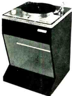
FAIRCHILD MODEL 750 —Three-speed 16" turntable handles LP's, 45's and 78's. Unique cueing pad for easy slip cueing, and torque characteristics of the drive system, allows startups from standstill in 1/4 turn (slip cue factor). The belt drive system allows turntable to be in a "ready" state at all times—no idlers to disengage or adjust. Noise-free to operate close to open DJ microphone. Available in black or new warm walnut.
