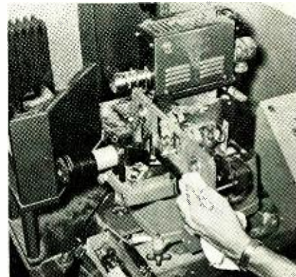
Fig. 6. Slide projector with cover off to show slide holders, lens, and gate.
