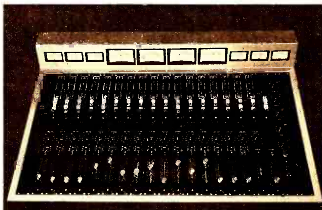
Close-up of modular strip design.
