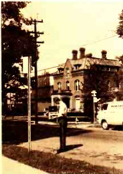
Fig. 1. Overhead wires are almost sure to result in false intensity readings.
