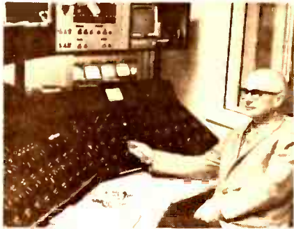
Fig. 2. Custom solid-state audio-control console was built by station personnel.
