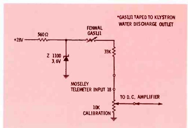
Fig. 14. Temperature problems detected with this circuit.
