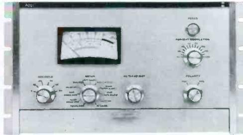
**900C Series Stereo Modulation Monitor.** Accurately measures and monitors FM stereo and mono programming in accordance with FCC Rules and Regulations. Removes all doubt about stereo signal. Fully transistorized.
