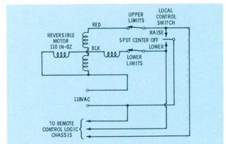
Fig. 6. Miniature switches limit motor rotation to 300° for power control.
