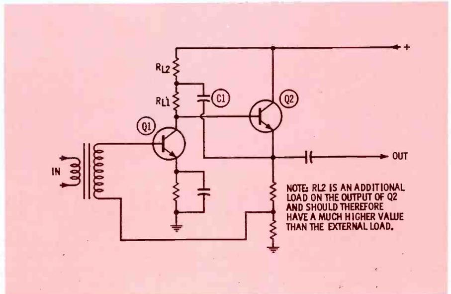
Fig. 3. "Bootstrapping" arrangement prevents partial loss of signal current.
