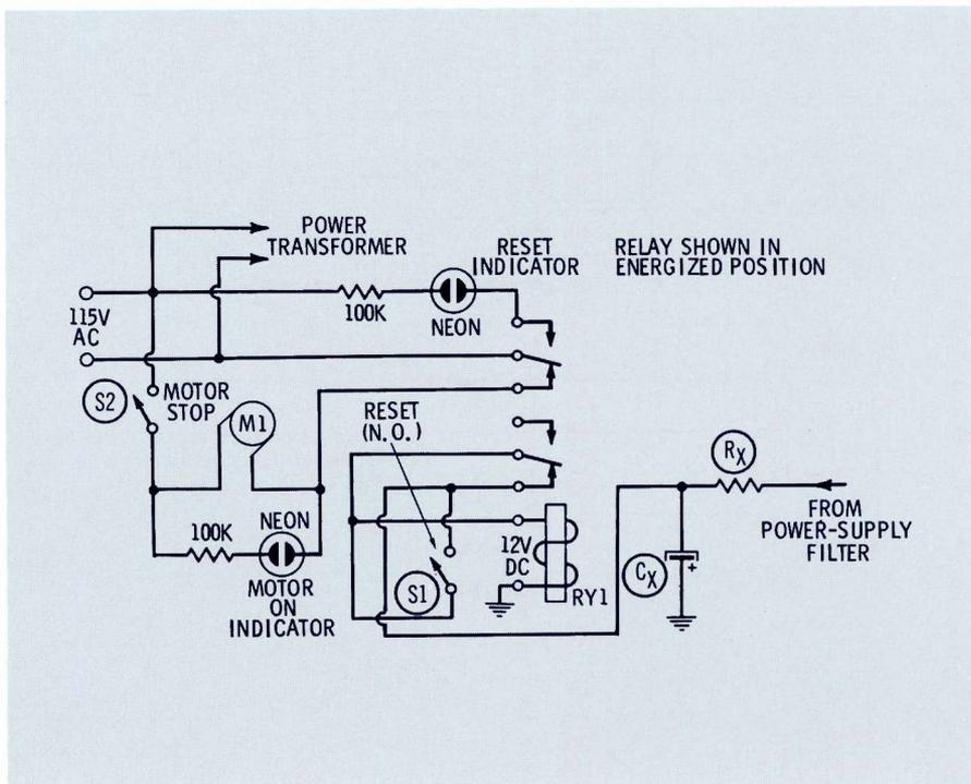
Fig. 2. Alternate failsafe circuit is insensitive to short outages.
