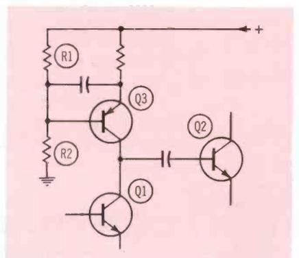
Fig. 8. Electronic choke replaces  $R_{L1}$ .
