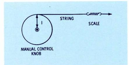
Fig. 5. Simple principle employed to determine motor torque requirement.
