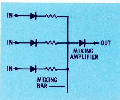
Fig. 10. Typical audio mixing method.
