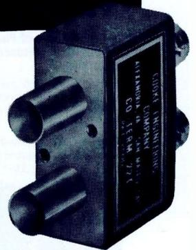
COTERM® provides the broadcast engineer with a new standard of dependability. With COTERM you have normal-through coaxial circuits without the use of patchcords. When the load side is patched the source is terminated automatically in the proper impedance.
