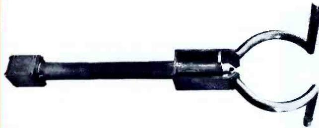
**37CP Circularly Polarized Antenna.** Electrical and mechanical design reduces dead weight and windload to a minimum. Does job previously performed by combination of vertically and horizontally polarized antennas. Cost about 30% less than combination arrangement. Fills in shadow areas, reduces null effects and improves fringe area reception. Design simplicity offers savings in new tower costs, erection time and maintenance.
