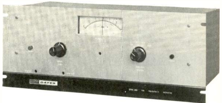
GTM-88F FM Frequency Monitor Wide-band pulse counting detector. No tuned circuits in pulse detector. All controls on front panel. Fully temperature compensated. Silicon solid-state circuitry.
