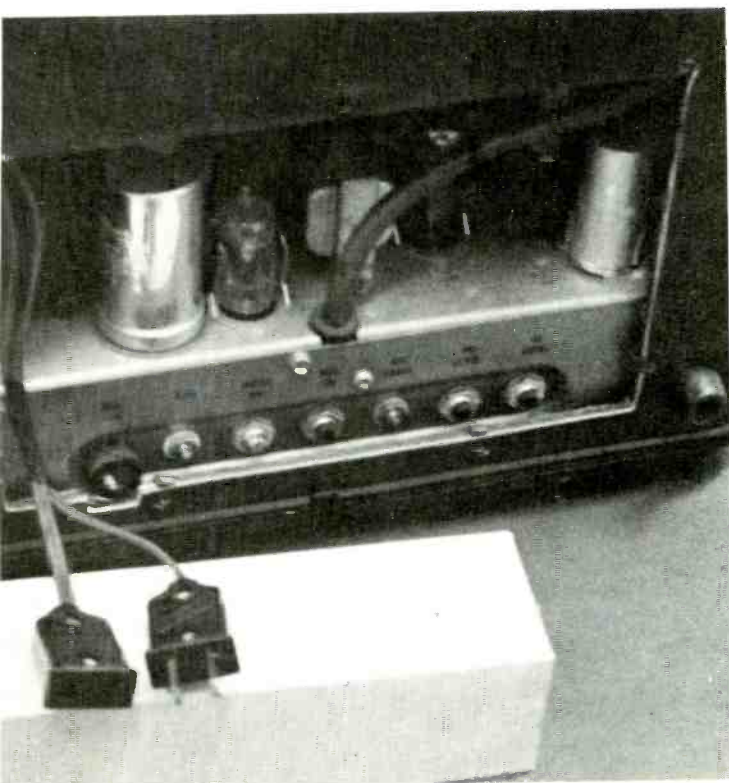
Fig. 4 Back of control unit shows control lines.
