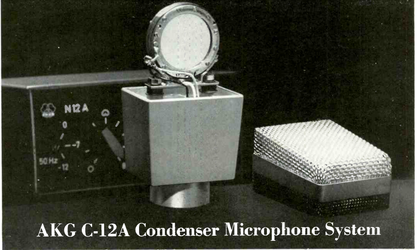
C-12A microphone shown with grille screen removed.
