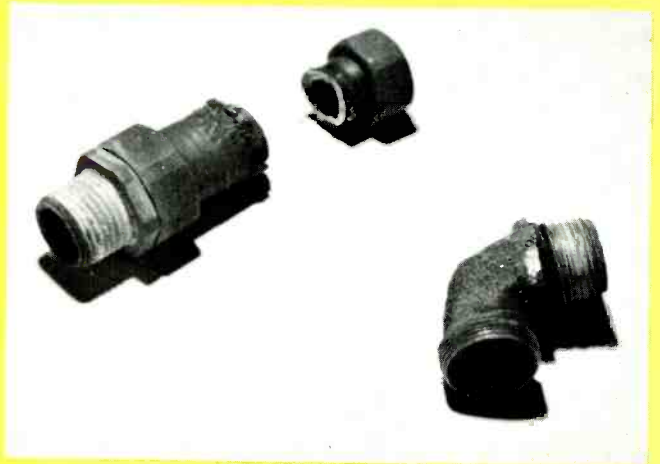
Fig. 3 Thinwall conduit wore enough to come loose from its compression fitting.
