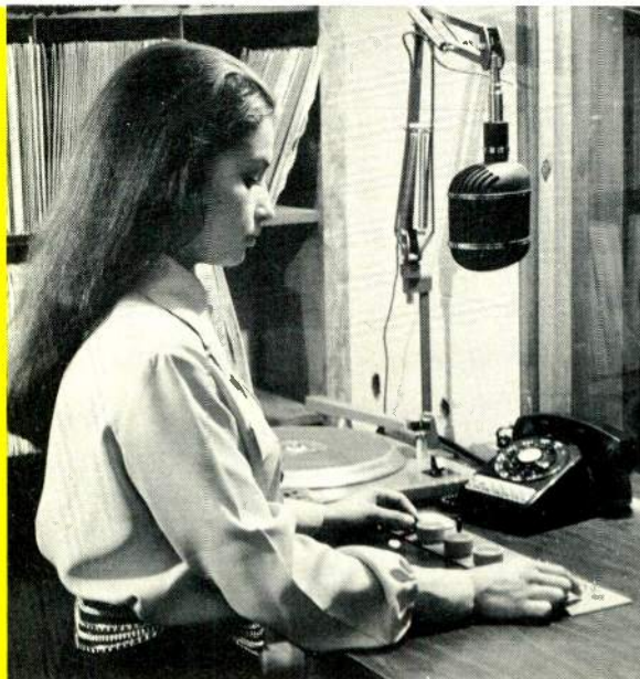
Fig. 1 Standup control board showing flush mounting.
