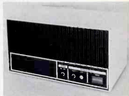
Fig. 2 The DIDS receivers will automatically deliver an alerting voice or teletype message to selected key locations or can sound a warning by sirens on command sent by unattended transmitters.
