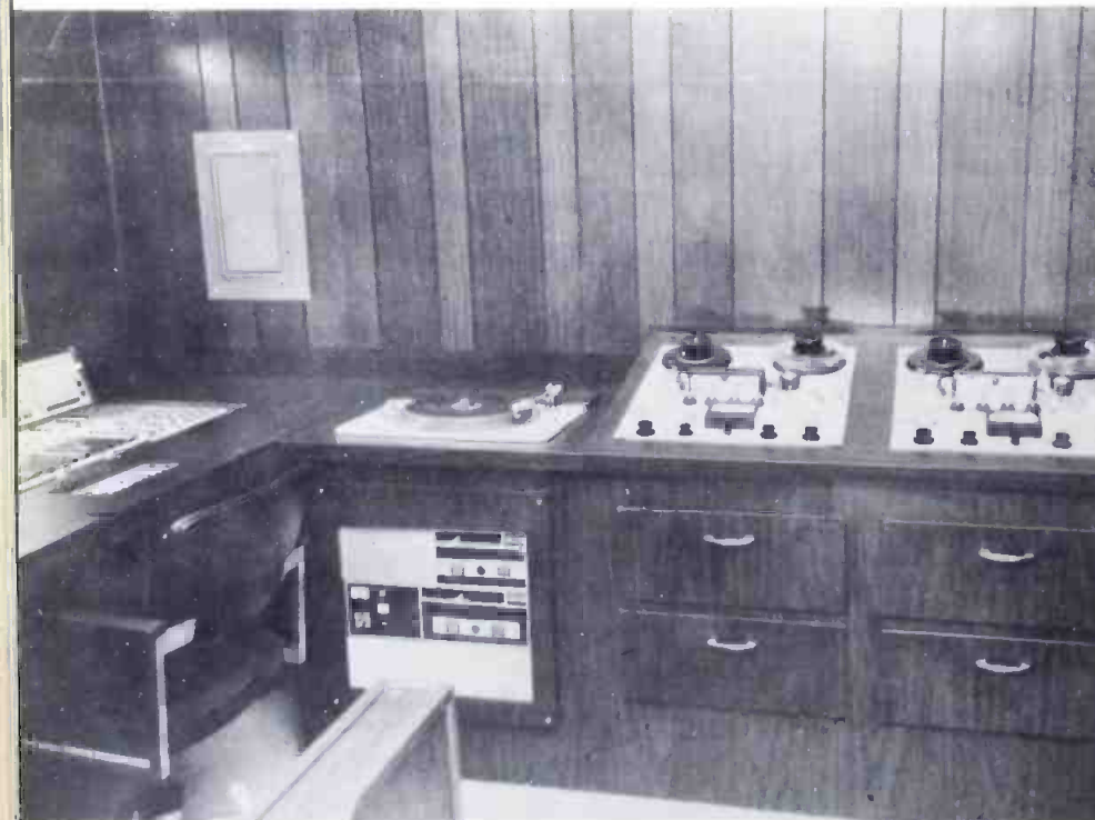
Fig. 7 Reel-to-reel audio recorders, turntable, audio cart machines and reverb unit are to the right of the console.
