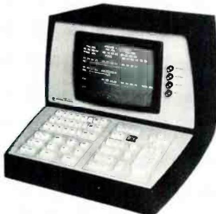
The system can perform combined audio/video, video only and audio only edits, and can be programmed to operate in conjunction with the Ampex HS-200 teleproduction unit.
