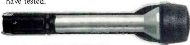
Let's look into the RE50 first. A cut-away shows that inside each RE50 nestles the familiar 635A, case and all. It's shock-mounted at top and bottom to the outer case. Even the connector is isolated from the actual microphone. And the problems
