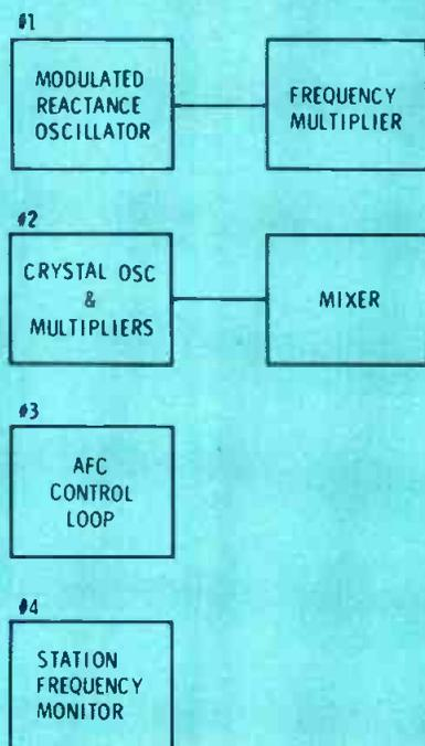
**Fig. 3** An off-frequency indication of the station frequency meter will be caused by one of these main divisions (aside from a blown fuse in the oven).
