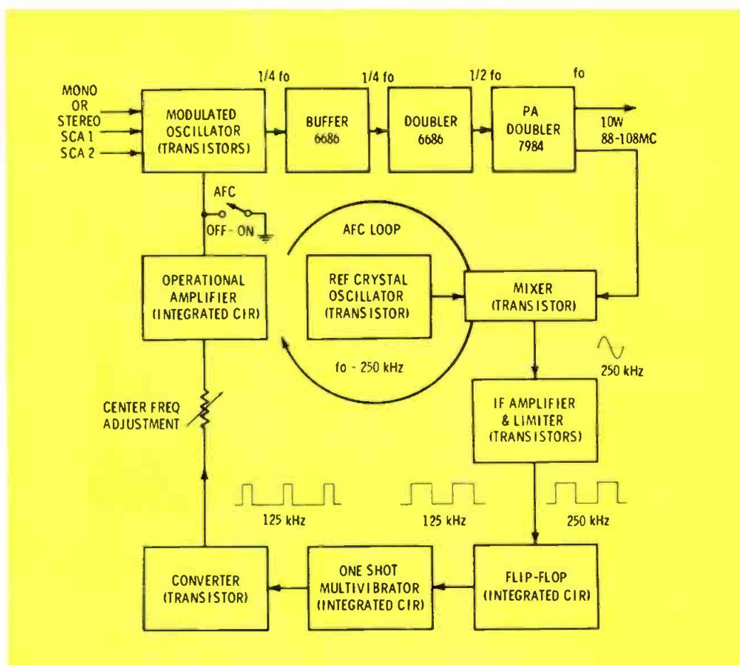
Fig. 2 New style reactance modulator exciter using a logic control circuit. This is a block diagram of the CCA Electronics FM-10DS.
