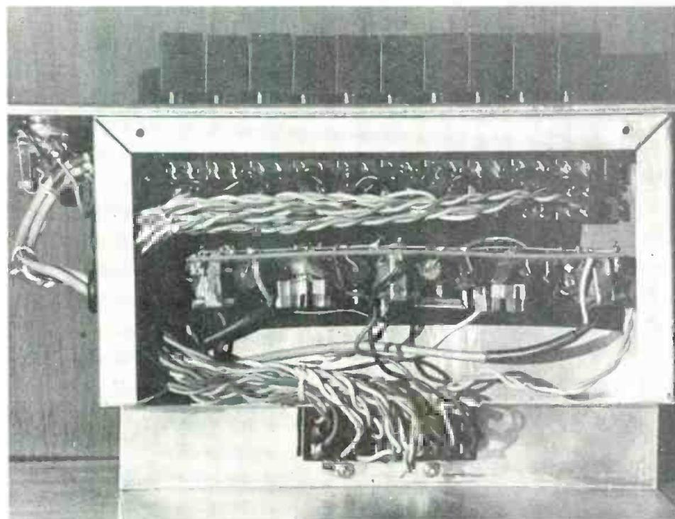
Fig. 2 Underside wiring of the headphone amplifier panel.
