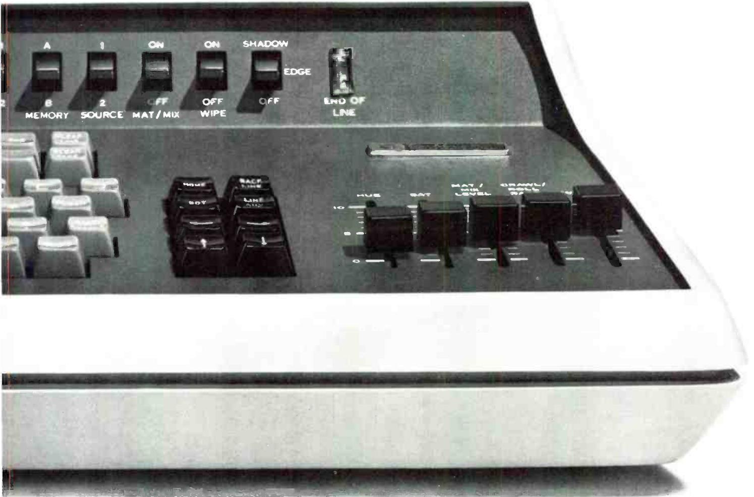
sponsibility. Built into the TCG-1425A is a solid-state switcher which permits selection between two video sources. The source selected is routed through the matting amplifier while the other source is bypassed through an equivalent delay circuit. One of the sources even has a fail-safe metallic-contact bypass.
