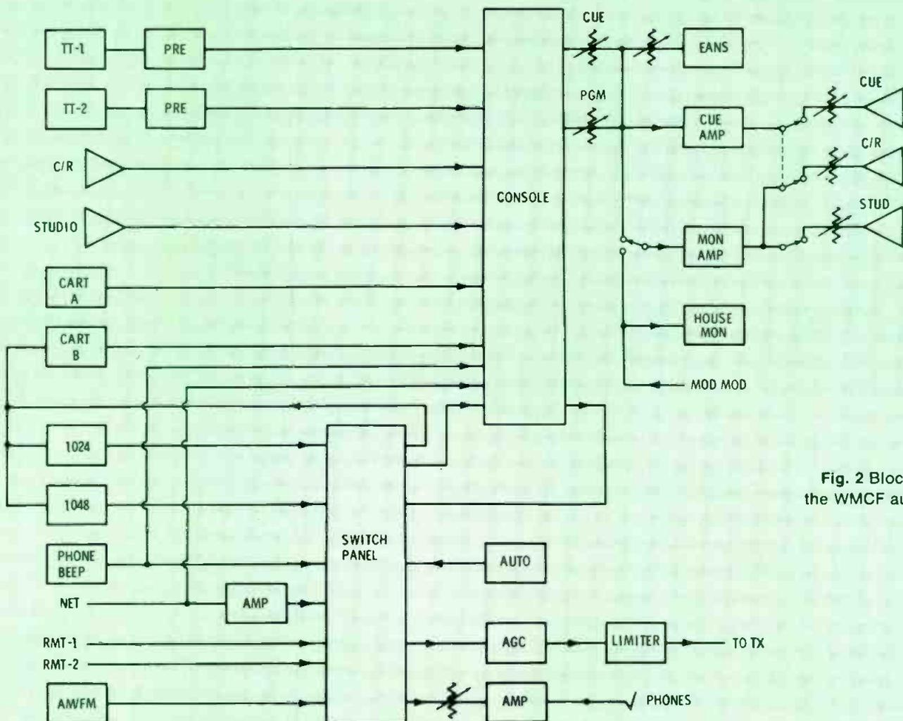
Fig. 2 Block diagram of the WMCF audio system.
