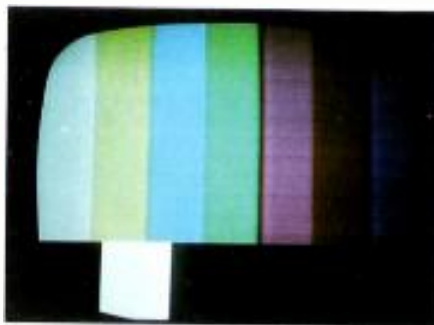
Fig. 8 Saturation banding due to a loss of response appears as a dark area within each band.
