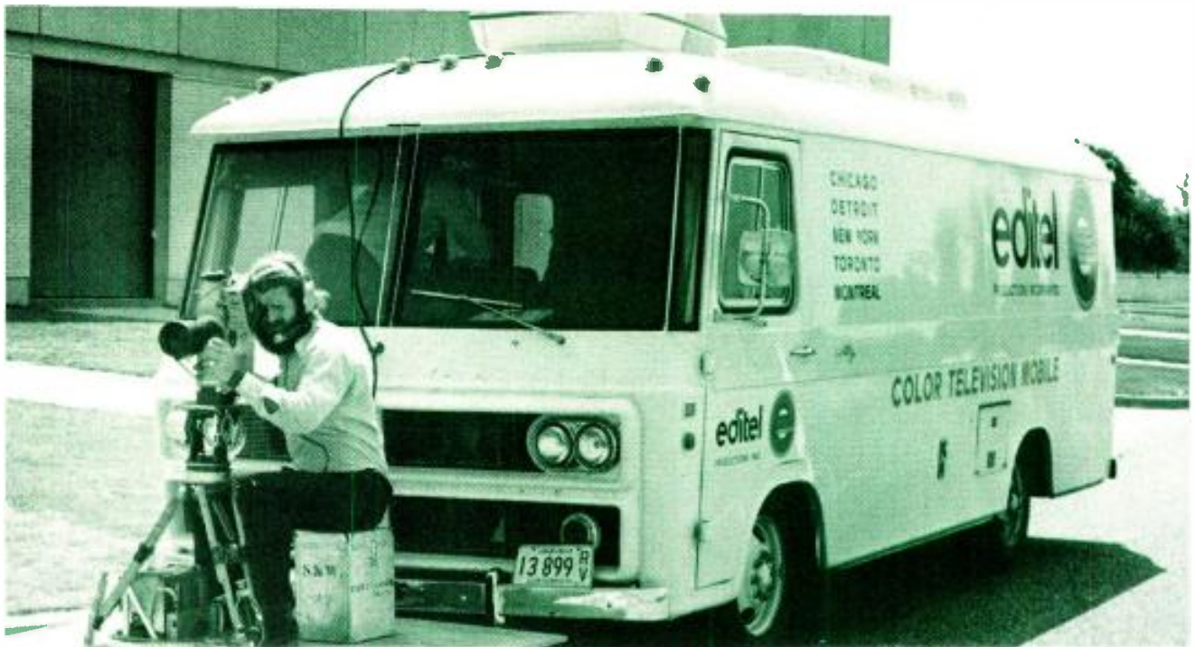
The Minimobile shown here at a remote site with camera operated from a special front platform.
