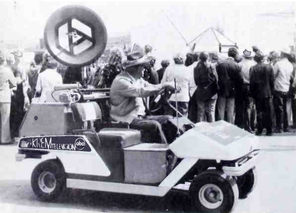
Fig. 1 The KREM LEM ready for action. Note that when the LEM is not in use, the microwave antenna is lowered.
