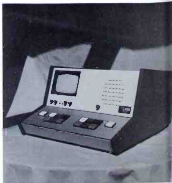
Fig. 1 The TRI EA-5 editing control system for helical VTR's.
