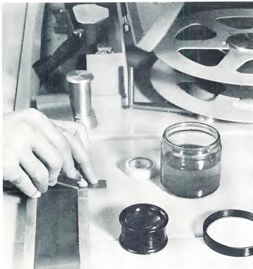
This was the earliest form of video tape editing using Edivue solution to locate the video tracks. The magnifying glass permitted easier viewing of the 10 mil tracks and the 5 mil guard band. After cutting with a razor, splicing tape was applied to the back of the tape.
