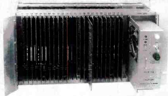
Starting with a single 8 $\frac{3}{4}$ -inch by 19-inch rack frame assembly, the user can build to a 20-input by 20-output configuration through selection of plug-in switching and amplifier boards.
