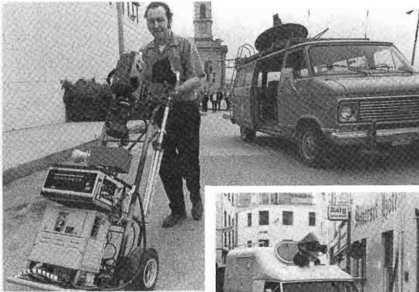
The "Batista Sling" at KMOX-TV on the scene with their version of a live news van. Note the dish is folded down for transport.
