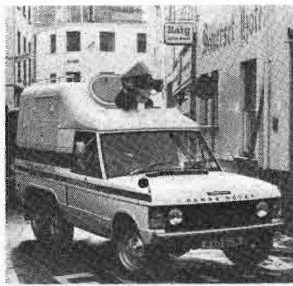
The Ranger Rover actually has three camera positions. Cameras can be mounted as shown (and operated while the van is in motion) or on the top or rear.
