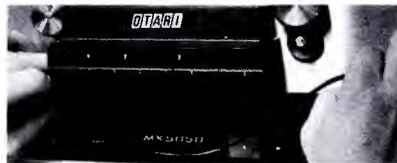
Easy threading, capstan on back side.
