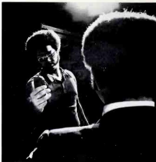
Figure 5 A footcandle or meter is an important aid in balancing the intensities of studio lights. Since dimmers affect color temperature, lighting directors now adjust not just intensity in three ways: altering lamp-to-subject distance; adding scrims; or, in the case of spotlights, pinning down the beams.
