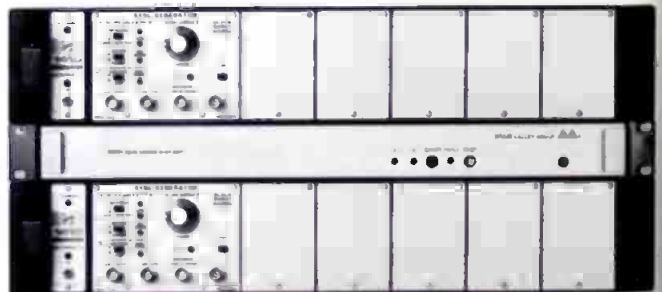
Typical NTSC sync generator system comprised of two 1410 Option 01 mainframes with SPG2 sync generator modules, and one GVG 3257A Automatic Changeover Unit.
