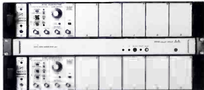
Typical NTSC sync generator system comprised of two 1410R Option 01 mainframes with SPG2 sync generator modules, and one GVG 3257A Automatic Changeover Unit.
