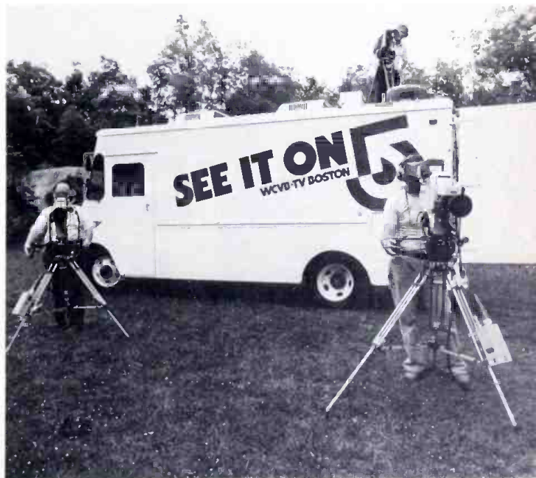
WCVB-TV engineers are pictured manning the three cameras of "The Hippo," a new, compact remote production unit. The roof-mounted RCA TK-76 joins two Ikegami HL-51s for unique production capabilities in a small, maneuverable vehicle.
