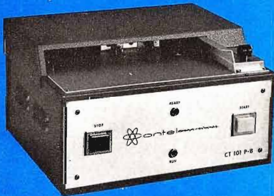
CONTEL model CT101P-B cartridge tape reproducer
