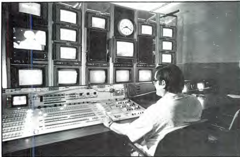
Independent productions benefit from the $2.5 million renovation that equipped the six KTLA sound stages with such equipment as this Grass Valley switcher in the Stage 2 control room.
