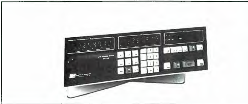
This CDL editor (EDS-200), introduced at the NAB convention in 1973, used the Intel 4004 CPU and appeared to be the first instrument for broadcasters and producers to use microprocessors.
