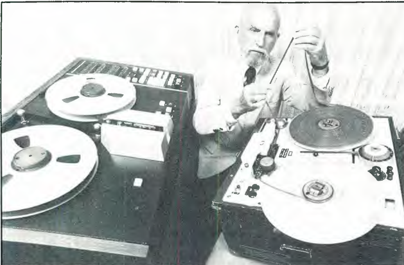
John Mullin checks his original red oxide tape on the Magnetophon which he modified to make the first taped U.S. radio network program by Bing Crosby in 1947. Here he was pictured at the 1978 AES Convention in Los Angeles, also flanked by the 3M 32-channel pre-mix digital recorder which utilizes a digital mastering tape developed by 3M.
