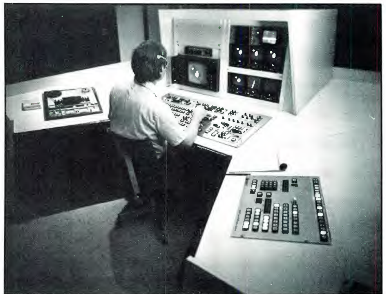
The master switcher control room with the microprocessor in the foreground, syncs up signals from CAESAR and SCANIMATE and routes them to the VTR room.
