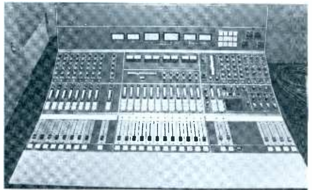
Figure 6 The control room 8X console is more complex than the air board but maintains a similar operational layout so that functions are easily learned.
