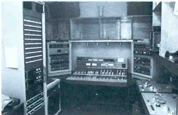
Figure 5 The WABC production control room 8X facilitates transfer of records and tapes to cartridges.
