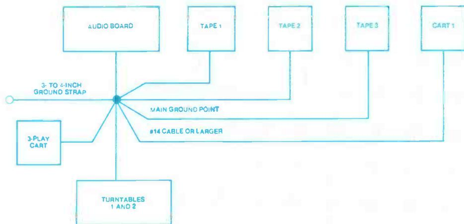
Figure 2. Ground system layout for individual equipment rooms.
