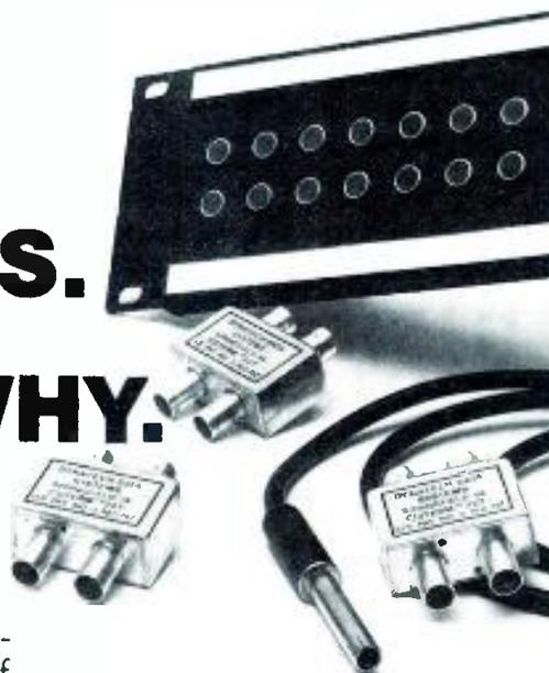
To Break The Normal-Thru Connection, you insert a patch cord that allows cross connections to be made. Sources that are patched-out are automatically terminated *within the jack in the proper impedance*. Test probes may be inserted in the jack to monitor a signal *without interrupting the live circuit*.
