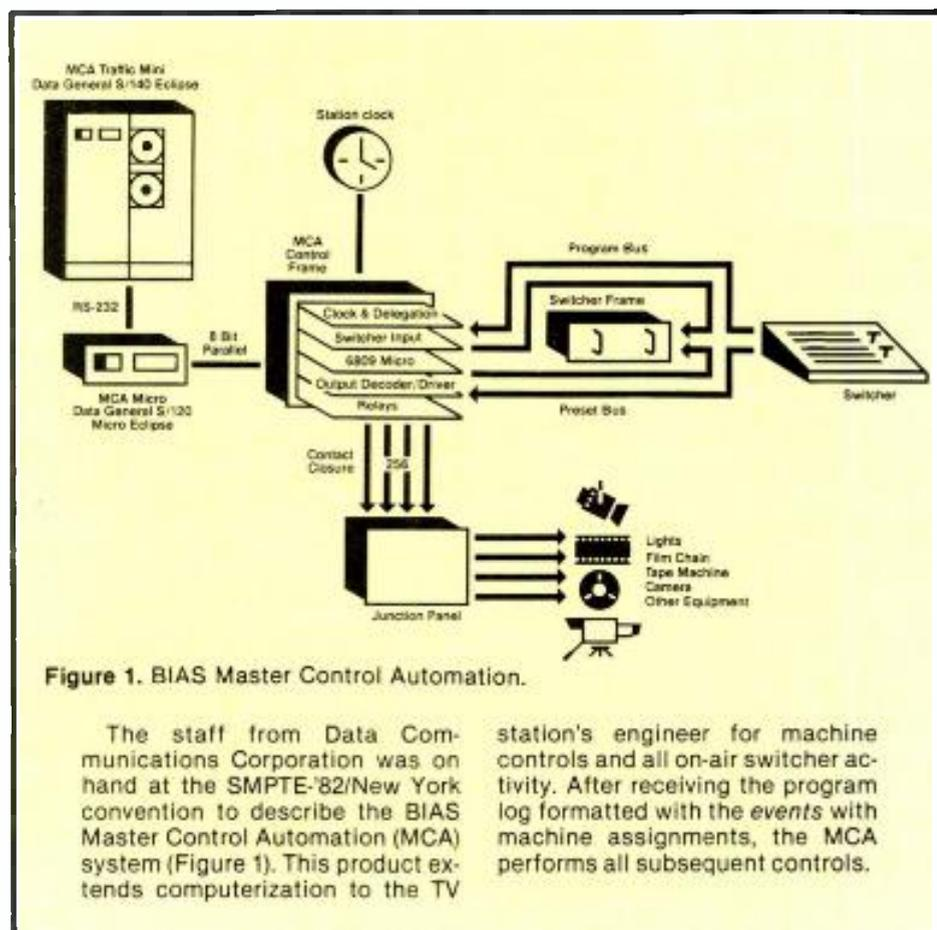
Figure 1. BIAS Master Control Automation.
