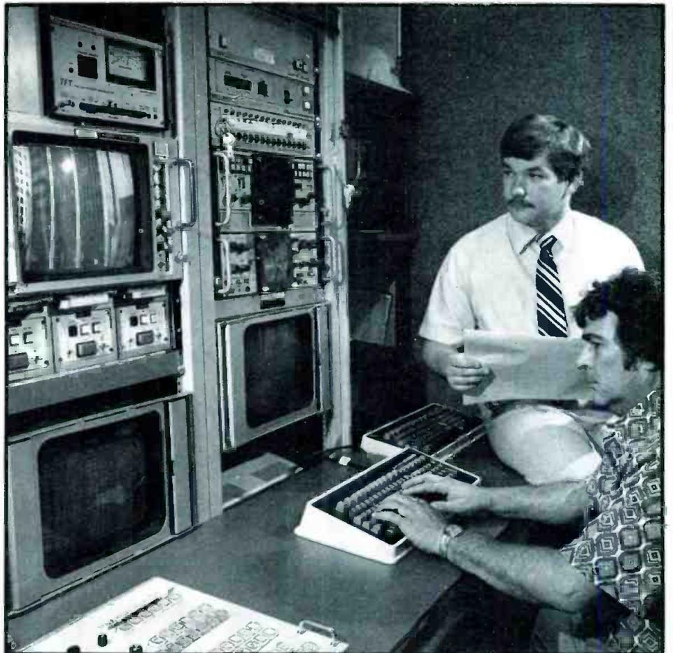
The WISH-TV automation system cuts on-air errors and improves billing. Charlie Clark (at the keyboard) demonstrates the log generating capabilities of the WISH automation system, while the author looks on.
