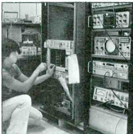
Each assembly level (module, chassis, final assembly) is subjected to test procedures before transfer to the succeeding assembly stage or inventory. Operating parameters are verified and documented before order processing and shipping.
