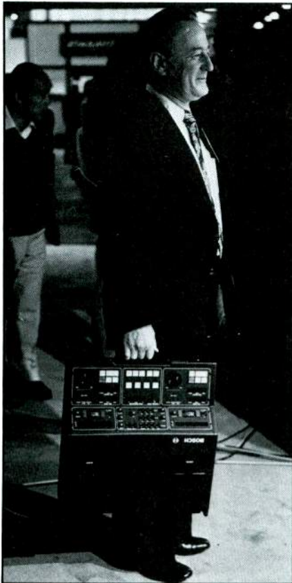
Henri Zahn with the Bosch 1/4-inch field editor that works with two 1/4-inch recorders from the combined camera/1-inch recorder unit.
