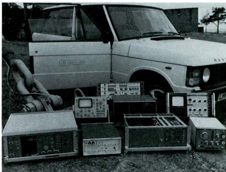
Shown is a full set of test gear currently carried by IBA transmitter teams for use at remote stations.
