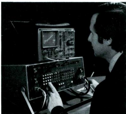
This Maintenance Automatic Test Equipment (MATE), developed by IBA engineers, replaces all the test equipment previously carried by transmitter maintenance teams.
