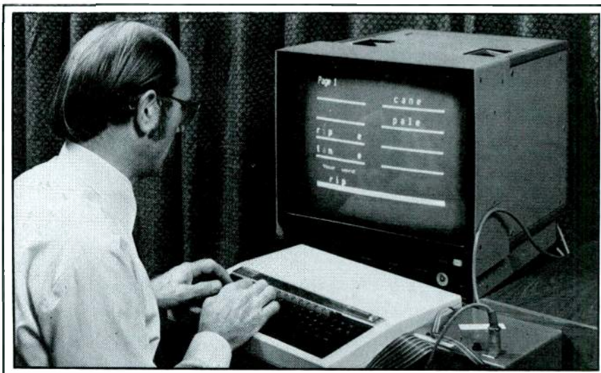
Shown are the BBC microcomputer and a teletext adapter that permits the direct downloading of software broadcast by teletext.
