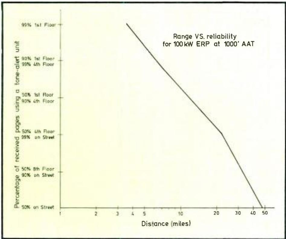
**Figure 2.** This graph plots range vs. reliability data received from the Seattle SCA tests. The transmitter power (ERP) is 100kW and the antenna height is 1000 feet above average terrain. Ten percent injection of the subcarrier is assumed. This chart applies only for tone-alert paging, which gives the greatest coverage range and is the predominant method of paging in use. The paging industry generally considers 90% reliability to be the minimum acceptable for most applications.
