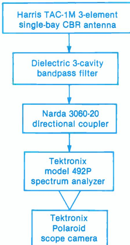
Figure 2. The Sears Tower receiving system used in the SCA experiments.
