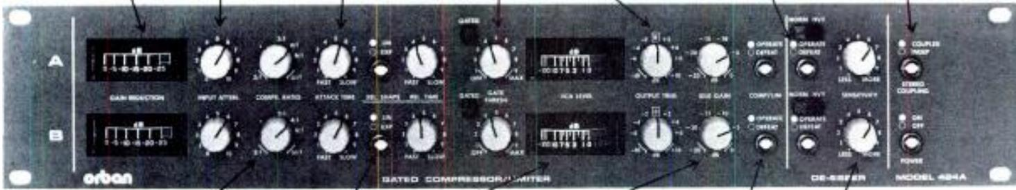
**GAIN REDUCTION:** Shows gain of the VCA (0 to -25db). Shows the effect of any control but OUTPUT TRIM and DE-ESSER.
