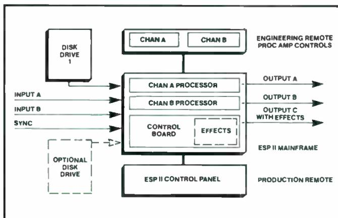
Picture quality is comparable with other ESP systems, as ESP II retains the 8-bit, 4-times subcarrier sampling scheme and, since the disk drive data format is the same as well, drives may be passed between systems or even shared in a dual-port configuration. Most popular disk drives can be used.
