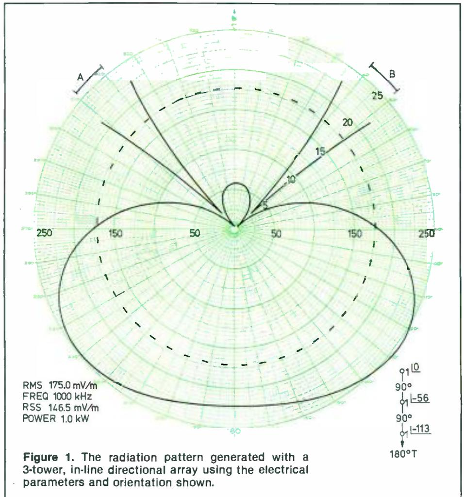
**Figure 1.** The radiation pattern generated with a 3-tower, in-line directional array using the electrical parameters and orientation shown.
