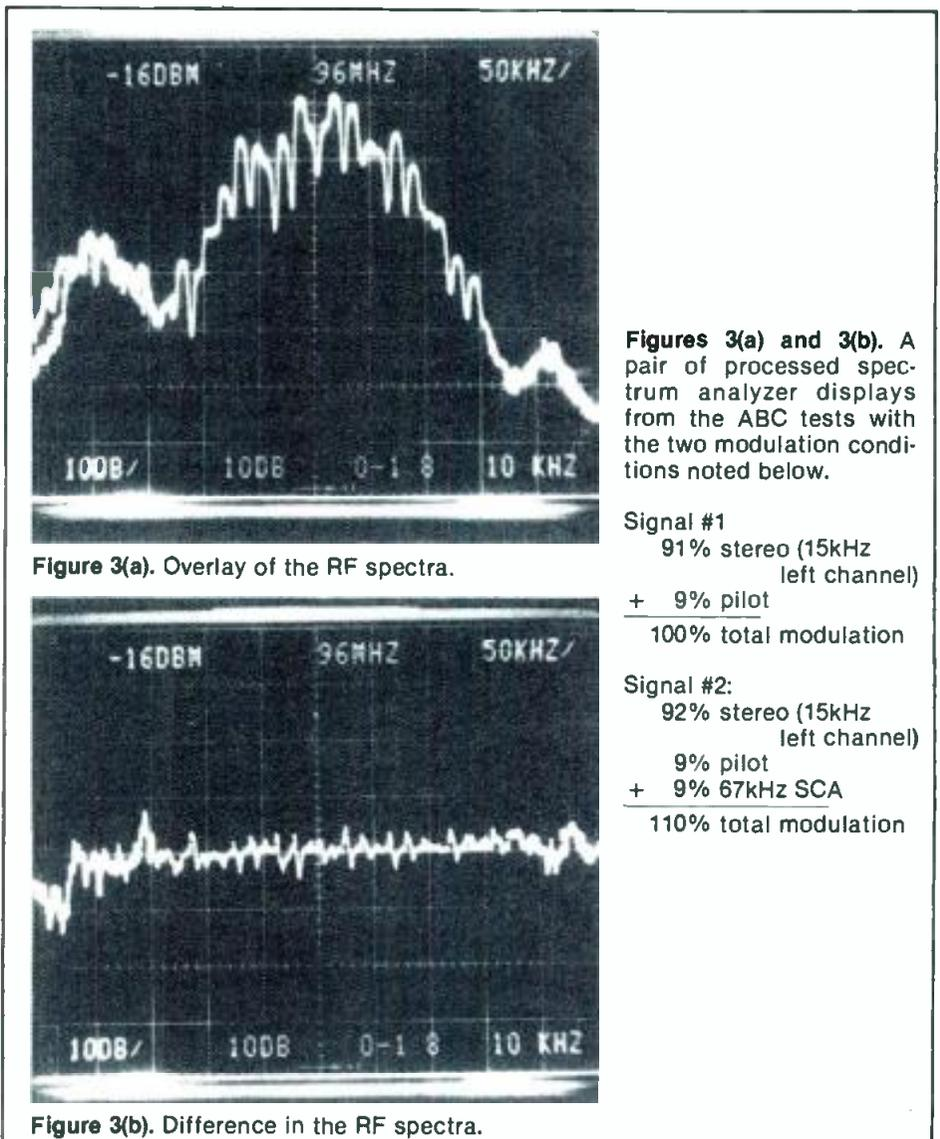
Figure 3(a). Overlay of the RF spectra.
