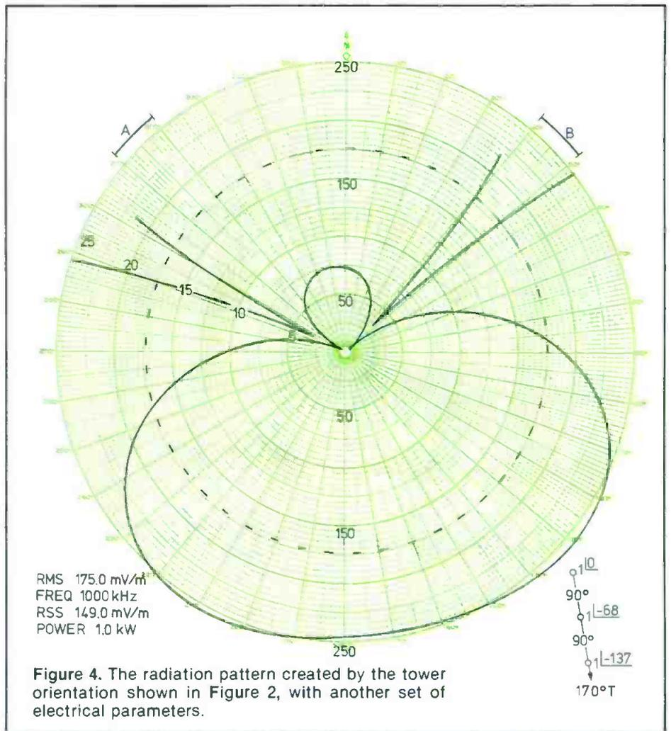
Figure 4. The radiation pattern created by the tower orientation shown in Figure 2, with another set of electrical parameters.
