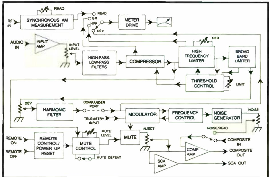
Figure 1. Block diagram of the Modulation Sciences Sidekick SCA generator system. The unit features remote-control capability and a compandor port for external processing of the transmitted signal.
