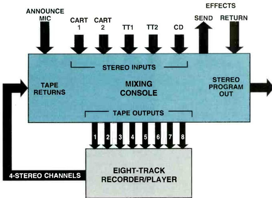
Figure 1. A traditional analog multitrack production studio configuration.
