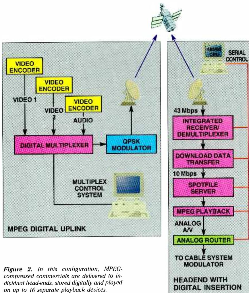
**Figure 2.** In this configuration, MPEG-compressed commercials are delivered to individual head-ends, stored digitally and played on up to 16 separate playback devices.
