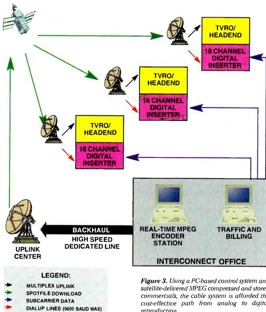
*Figure 3. Using a PC-based control system and satellite-delivered MPEG compressed and stored commercials, the cable system is afforded the cost-effective path from analog to digital reproduction.*
