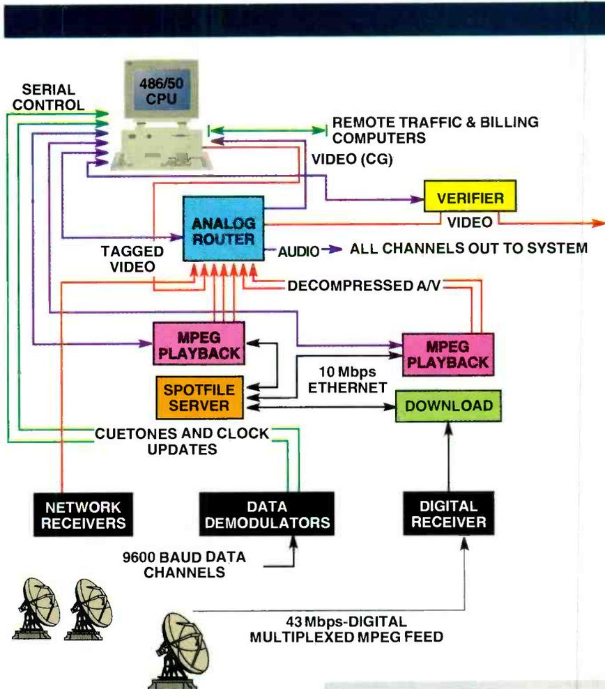
**Figure 1.** Digital satellite delivery of commercials can tie even the most remote cable systems together as an interconnect, or transport national and promotional spots for near immediate turnaround.
