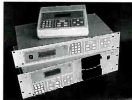
• **Timecode Monitor**: used for fault-finding, confidence reporting and unattended monitoring of SMPTE/EBU longitudinal time code; can simultaneously monitor, analyze and report errors in vertical interval time code (VITC).
