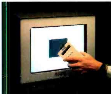
• **CODES:** handheld, lightweight testing device designed to provide an easy check for electronic display degradation of an installed system in its working environment; operator can complete a performance evaluation of an electronic display and make spot decisions on a CRT in just a few minutes.
