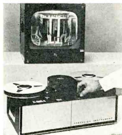
degree of slow motion, or with motion stopped completely. The equipment, designated PI-4V, incorporates Variscan playback speed control, continuously variable from stop to normal speed. Using 1" tape and two audio tracks which may be individually erased and re-recorded, the completely transistorized PI-4V is said to be as simple to operate as home audio tape recorders.
