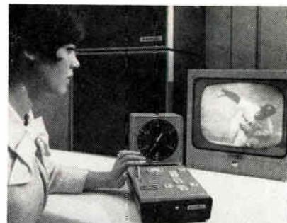
metal discs instead of magnetic tape, is capable of instantaneous replay of televised action at normal, fast and slow speeds down to frame-by-frame stop action. Its capabilities also include reverse action playback or analysis of highlights.
