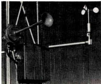
of Sunnyvale, Calif., consists of a wind speed sensor, an electric transducer and an electric warning horn. The unit may be set to trigger alarm at any speed from 1.5 to 120 mi/hr  $\pm 2$  percent for protection of radio towers. Unit operates on 115 V ac. Circle 101 on Reader Service Card
