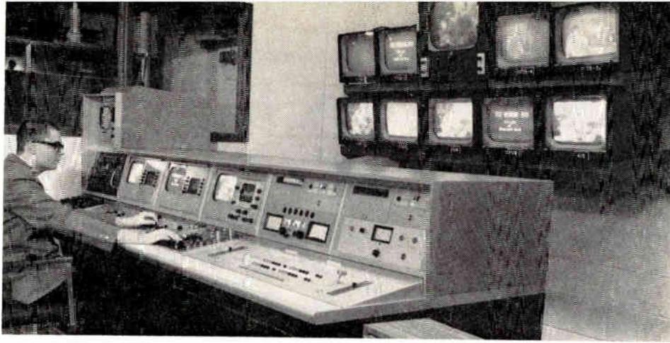
Closeup view of the master control console. Transmitter meters are visible to the engineer on duty.
