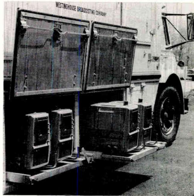
Fig. 6. Storage area of van shows camera storage, camera accessory storage and cable reels.
