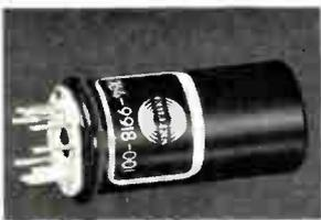
**Photocell Operation.** The photocell lamp completely isolates control voltage from the audio circuits for audio switching and level control. Small physical size enables the photocell to be located in active audio circuitry, thus keeping audio leads to a minimum. Switching time constant eliminates transients such as pops and clicks.
