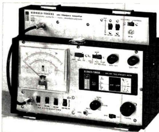
Look twice—Blonder-Tongue's new model 4132 sub-channel converter is shown mounted on company's FSM-2 field strength meter, booth 21.
