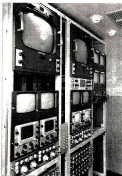
Fig. 3. Operating panel for video technician shows two cameras per 19-in. rack.
