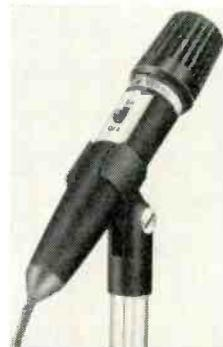
Model 2850 miniature, dynamic cardioid microphone weighs less than 3 oz. and may be used in the hand, on a stand, or as a lavalier. Unit is six-in. long, has a head diameter of 1-13/16-in., has a housing molded of tough Cyclocac and has a 70-12,000 Hz frequency response range. At high impedance, the output level is -60 dB; at 150 ohm impedance output is -62 dB. Microphone is supplied with a 12-ft cable. \$40.00. The Turner Co.
