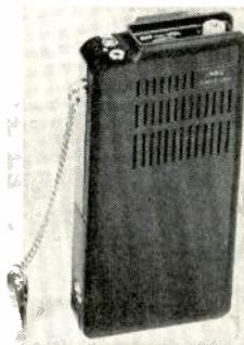
Model PR-150/2 fm selective-calling, solid state paging-receiver operates in recently FCC-assigned 150 MHz band as well as in 30-50 MHz band. Weighing 7 oz., the receiver measures 2½ W × 5 H × ¾ D in. The crystal-controlled double super-heterodyne receiver offers either beep-only or beep-plus-voice and is available for operation with rechargeable batteries or dry cells. Price is under \$200 and delivery is about 120 days. Minilec Devices, Inc.
