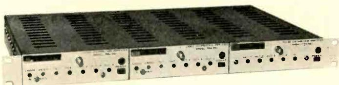
TeleMation's TMV-551 Video Distribution Amplifier provides four completely isolated outputs from one bridging input. Built-in power supply and connector panel, IC series regulator for constant power supply voltage standard. Top color performance.
