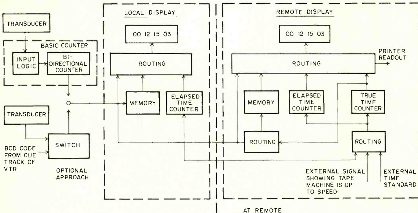
Figure 3. Block diagram of counting system.
