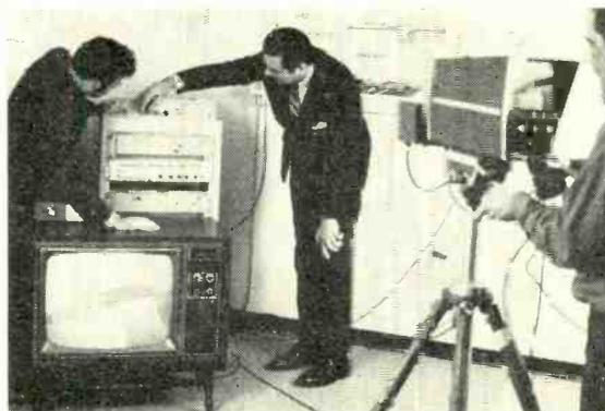
All of the elements of the Athena cable TV encoder-decoder system. Encoder precedes the headend signal processor.
