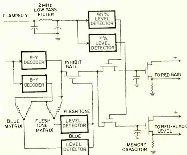
Fig. 4. Automatic film color balance
