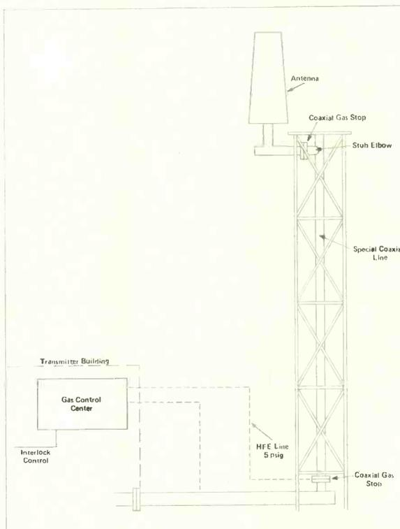
Diagram of a transmission line using dielectric gas.
