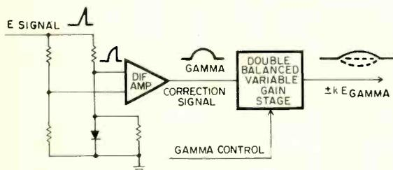
Fig. 3. Gamma error correction signal
