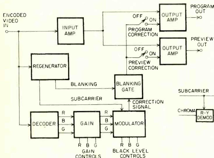
Fig. 1. Encoded signal color corrector
