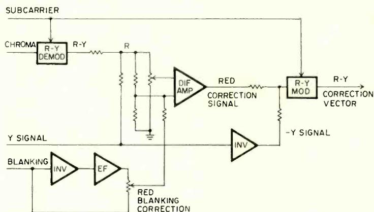
Fig. 2. Red correction channel
