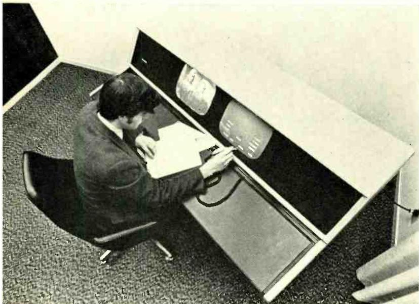
CMX 600 permits easy editing and assembly of film. After assembly correction factor can be entered before recording on tape.
