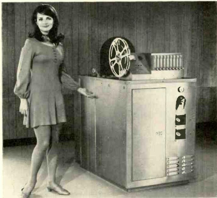
**CCTV console, camera** are designed for compact portability, remote use. Originator II console is desk-top portable including EIA RS-170 sync generator, six-input switcher-fader with preview bus, vertical interval switching, audio mixer, video monitors. TVC-625 vidicon camera has 850-line resolution, 60-gauss field, FET hybrid cascade input amplifier,
