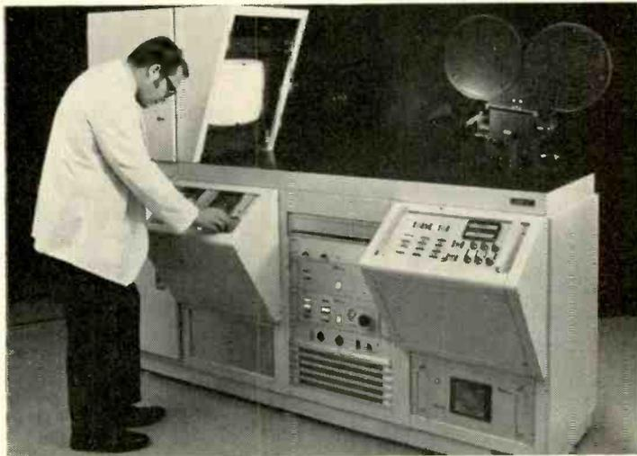
**Color video film recorder Model CTR-2** features high-resolution tri-color kinescope, H and V aperture equalizers, comb filter decoder for chrominance/luminance separation, vectorscope, photometer, 10-step gray-scale generator. Camera is 35-mm with  $f/1.3$  lens, driven by closed-loop phase-locked system using air bursts for film advance. Suitable for both negative and reversal color film; scan reversal available. \$75,000. TELEDYNE CAMERA. **290**
