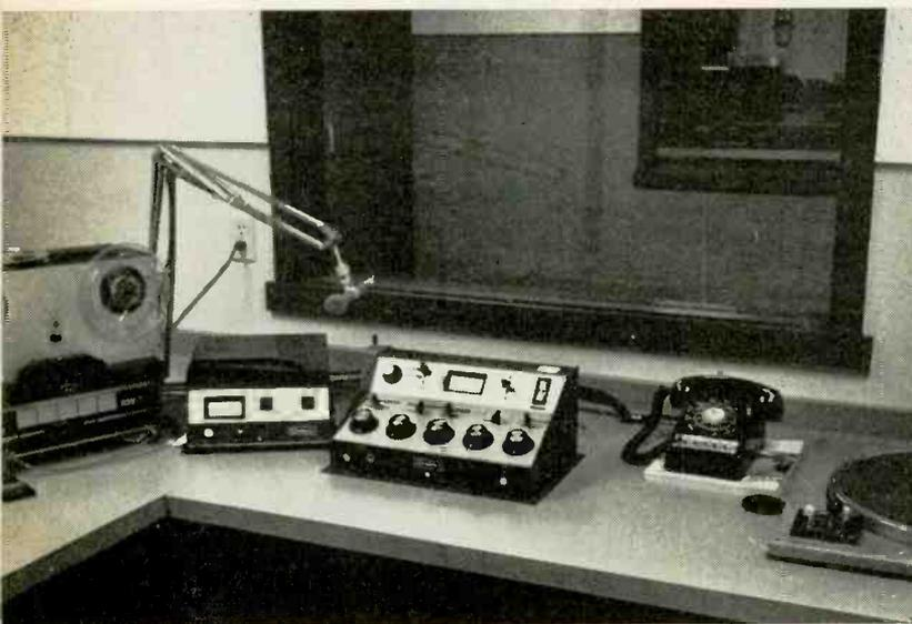
New production room at KVEC is still small, but more efficient use of space has been made. One space-saving feature is solid-state Sparta equipment. Window looks into center studio where recording or live broadcasts originate. Beyond that is control room. All three rooms are temperature-controlled and soundproof.
