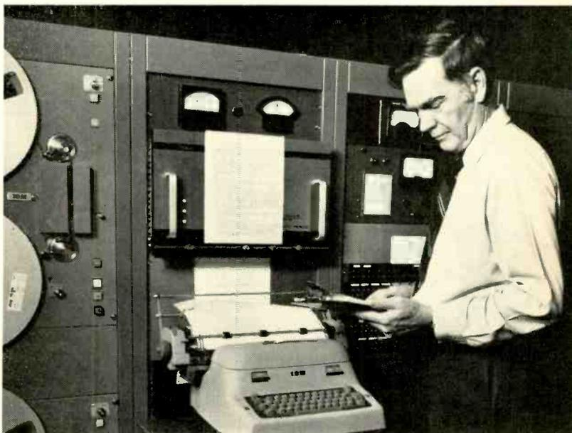
WFIR Chief Engineer E. F. St. Clair checks readings on the Moseley automatic logger, and reviews correctness of signatures on the cover sheet attached to each day's log.
