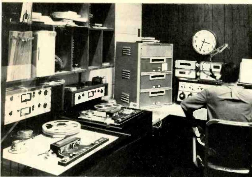
Production studio at WFIR includes two Gates turntables (not shown) plus reel-to-reel and cartridge tape equipment. Under clock are remote controls for automation, cart encoding, and audio control.
