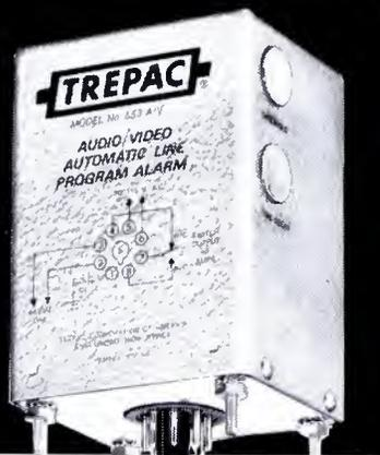
TREPAC MODEL 553 A/V AUDIO/VIDEO AUTOMATIC LINE PROGRAM ALARM senses variations of signal level, and provides automatic control of alarm or other associated equipment. It eliminates the need for continuous personal attention. The unit is activated whenever the audio or video line program level deteriorates below a preset threshold.
