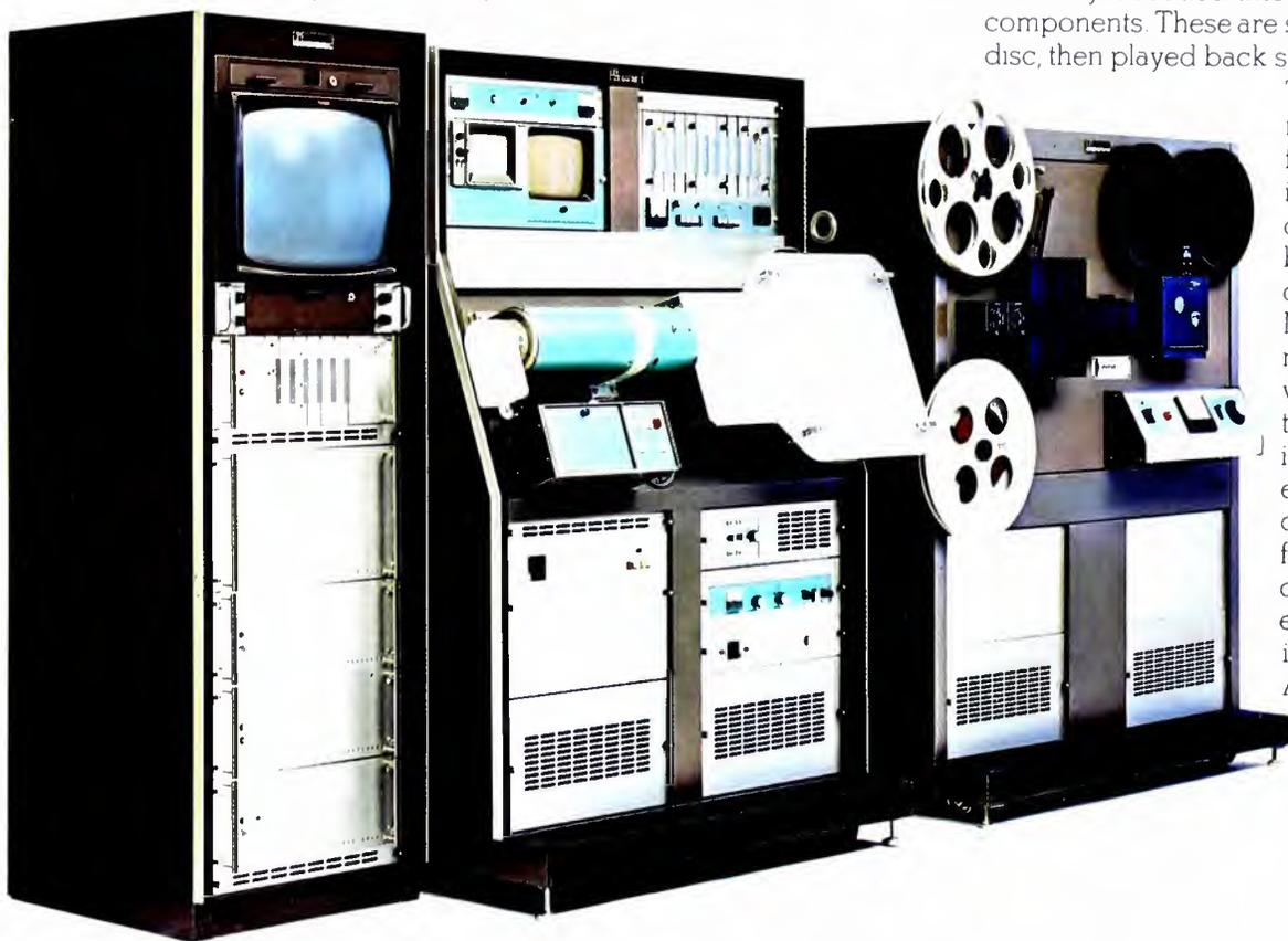
Waveform monitor permit the operator to electronically make all necessary video adjustments and calibrations prior to recording.
