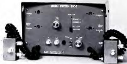
switching rates are 0.2 to 200 Hz; internal sync, 5 to 100 Hz. 75 or 50 ohm input: BNC, TNC or F connectors. \$260.00. KAY ELEMENTRICS CORP. **299**
