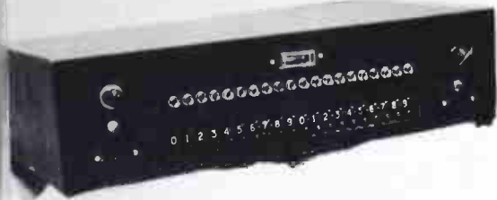
Thumbwheels set up the sequence of sources that will be automatically connected on the Smith automation unit. Light indicates which source is operating.
