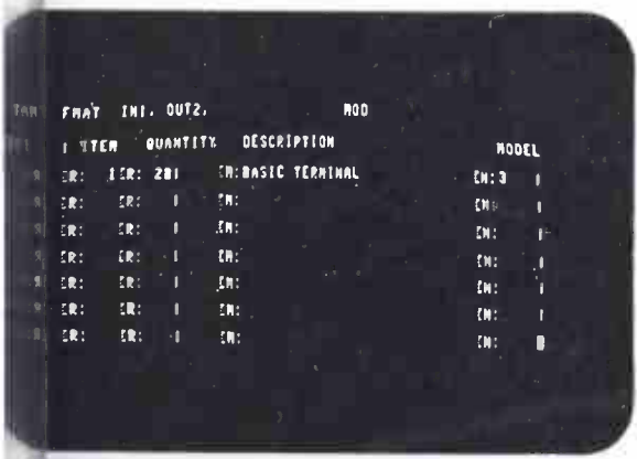
The next page of the format program defines the Order. Note that an incorrect character was typed into the Model field which the terminal has accepted. The error message, MOD, is displayed, an error alarm sounds, and the keyboard
