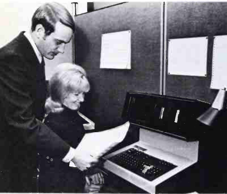
Mini-computer used "on location" in Jefferson Data's "System 80" is the Sycor 340B. Entire unit can be seen on table top, at lower right in photo. CRT display screen, on which entries can be read before insertion in memory, is at left end of upper panel. Cassett tape memories are inserted at right of upper panel. Keyboard includes alphanumeric keys plus function keys, and is entry not only to mini computer but to main computers, via telephone line.
