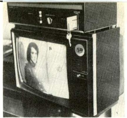
Above: plastic card attached to room key is inserted in set-top converter to unscramble movies, activate security sensors. Below: info readout for hotel administration.
