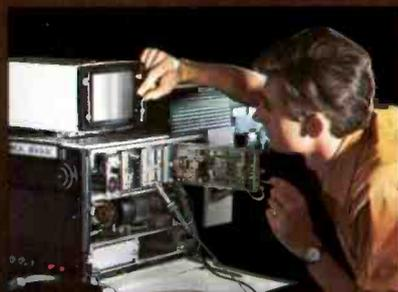
**Downtime virtually eliminated. Instantly-accessible plug-in circuit boards can be changed in seconds. No trouble-prone multi-layer circuit boards.**
