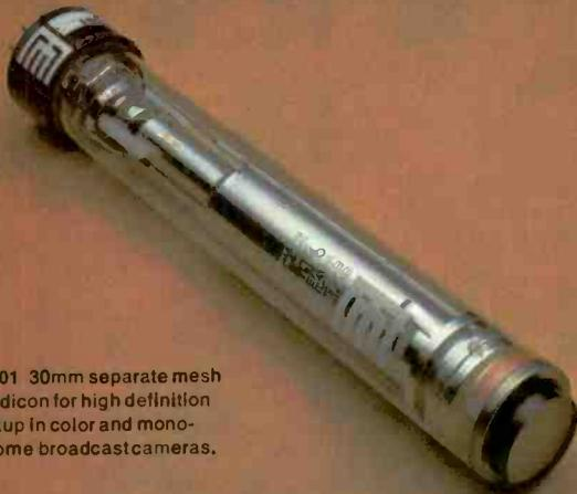
P8001 30mm separate mesh Leddicon for high definition pickup in color and monochrome broadcast cameras.
