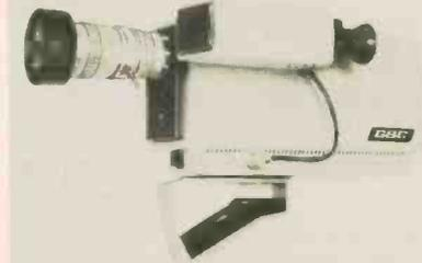
a 1½-inch viewfinder, Model CTC-5X, features built-in automatic sensitivity control. It also has a front panel trigger switch for activation of portable VTR, an adjustable control for outdoor or indoor shooting and EIA RS-170 sync. \$2,000. GBC CLOSED CIRCUIT TV CORP. **303**
