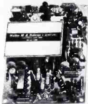
is above 2,000 ohms and output impedance is 50 ohms. Dynamic range is 47 dB; differential phase is 0.5° and differential gain is 1%. WALTHER M.A. ANDERSEN & ASSOCIATES 316
