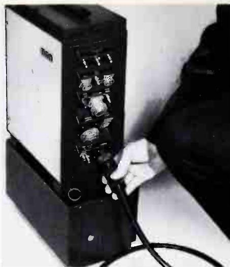
replaceable in seconds. Where AC current is available, a plug-in adapter can be substituted for the battery pack.
