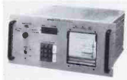
or elsewhere. The Series 5300 provides graphic performance monitoring, showing cable system performance at each of monitored points, with hard copy available. Central analyzer, \$3500; each remote monitor, \$800. **INTECH LABORATORIES 312**
