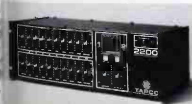
equalization bands. Model 2200 provides boost or cut up to 15 dB on each band; built-in line drivers allow interface with hi fi equipment or low-level mixing systems. Both input and output have transformer balanced or unbalanced connections. Distortion is rated below 0.06% at 10 volts output, SNR at better than 80 dB. \$289.00. TAPCO 302
