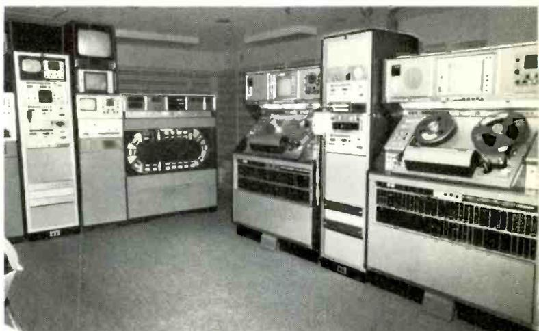
"cart" machine is used for filling in a "doughnut" commercial. After the intro, an action clip from the film might be inserted, with a part of the sound track, or a voice-over announcement. Using the A to B external dub mode on the TCR-100, the intro and extro material is played on the "A" deck through the switcher, where "fill" material is inserted, with the composite being recorded on the "B" deck.
