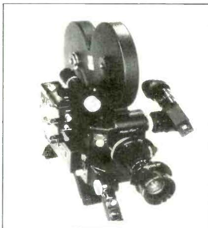
zoom lens; 400 ft. Frezzi/Mitchell magazine; film load; quick-change internal nickel-cadmium battery; Frezzi MCA-16 two channel side-mounted amplifier; sound head; "street" weight is 16½ lbs. Design permits quick plug-in installation of a side-mounted amplifier for single-system sound operation without ex-
