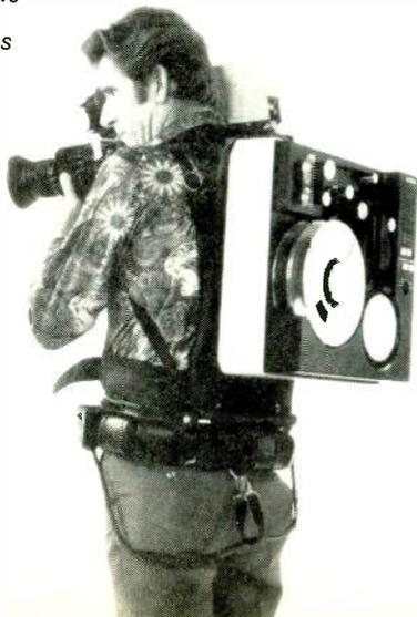
VPR-10 as backpack creates completely portable recording system.
