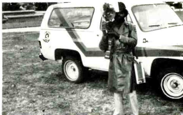
ENG Type II vehicle is rugged 4WD Blazer. Has no built-in gear except two-way radios and battery chargers.
