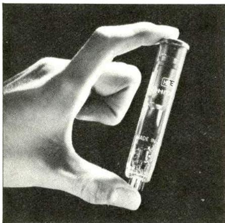
The Hitachi SATICON, a newly-developed camera tube, is characterized by heterojunction target between tin-oxide and selenium doped with arsenic and tellurium in its photo-conductive layer.
