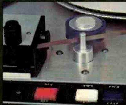
"This new high-friction polyurethane roller pulls the tape with less pressure. Less wow and flutter."
