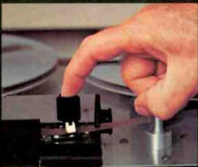
"There's also a fool-proof push button tape marker. Or, I can crease-mark the tape against a disc positioned for this purpose."
