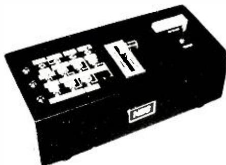
Standalone control panel (incorporates an A/D converter) interfaces the digital video processor to the switcher.
