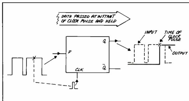
Fig. 3B. A flip-flop is clocked.
