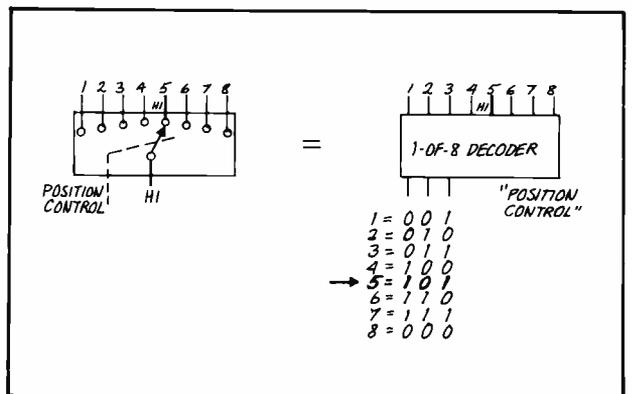
Fig. 9. "1 of n" decoder as selector switch.
