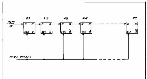
Fig. 4. Flip-flop formed into a shift register.
