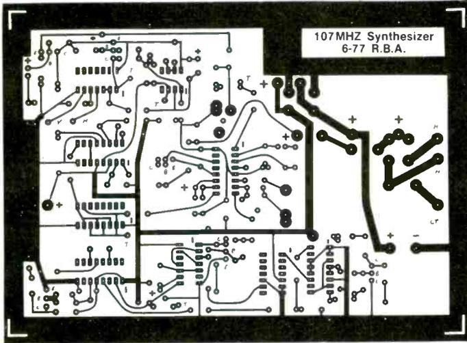
Underside shows circuit connections on Allen's synthesizer board.
