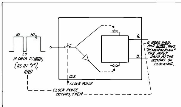
Fig. 3A. Flip-flop extended to remember data.
