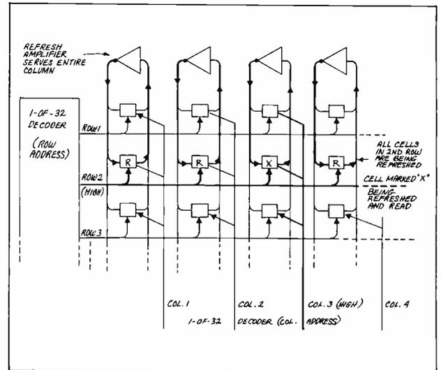
Fig. 14. System requiring only 32 refresh amplifier.
