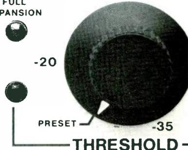
Program-controlled filter suppresses residual background noise in audio reproduction systems. Selectable low frequency, high frequency, or wideband suppression modes.
