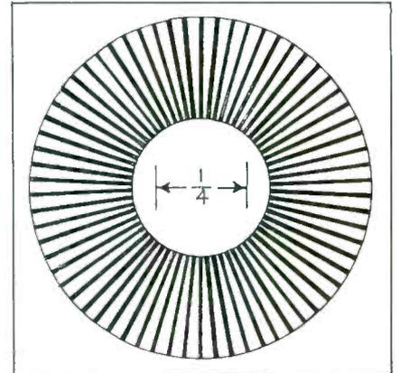
**Solution:** Construct a strobe disk which can be mounted to the front of the sound drum with rubber cement or
