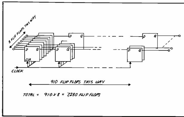
Fig. 5. Shaft register organized to handle 8-bit system.
