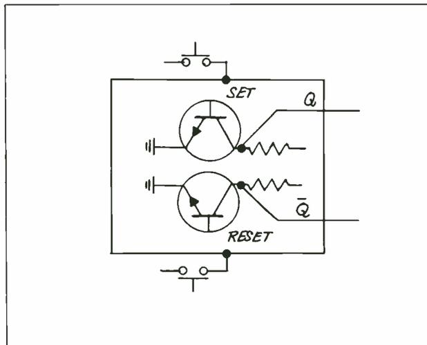
Fig. 2. Flip-flop with two outputs.
