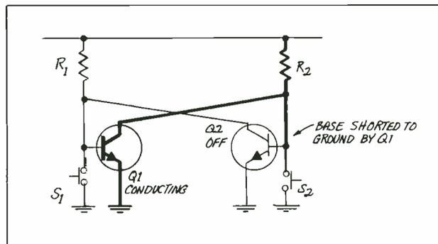
Fig. 1. Simple flip-flop circuit.
