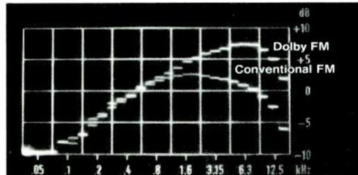
Real-time analysis of Dolby FM receiver output when tuned to interstation noise, using Altec Hewlett-Packard 8050A analyzer. In a "perfect" FM system the trace would be a continuously rising straight line. Thus the results show that highly modulated high-frequencies can be reproduced with significantly improved accuracy using Dolby FM.
