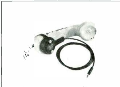
microphone). The telephone mouthpiece is not removed, nor is telephone wiring system altered in any way; unit has no induction coils. Background noise is eliminated by complete coverage of mouthpiece. A lever allows interjection of live commentary without interrupting transmission of the taped material. Unit has a frequency response tailored to 300 to 3000 Hz for optimum voice transmission via the telephone. \$28.50. SHURE BROTHERS.
