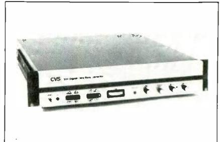
PAL is corrected composite video; for SECAM it is synchronized RGB that can be routed to an RGB switching system. The unit can also act as a PAL/SECAM converter with a plug-in SECAM option. Thus either PAL or SECAM in can be PAL or SECAM out. Unit has genlock signal generator; color dropout compensation; line by line velocity compensation; digital color averaging; a processing amplifier; and a 2-line window. CONSOLIDATED VIDEO SYSTEMS.
