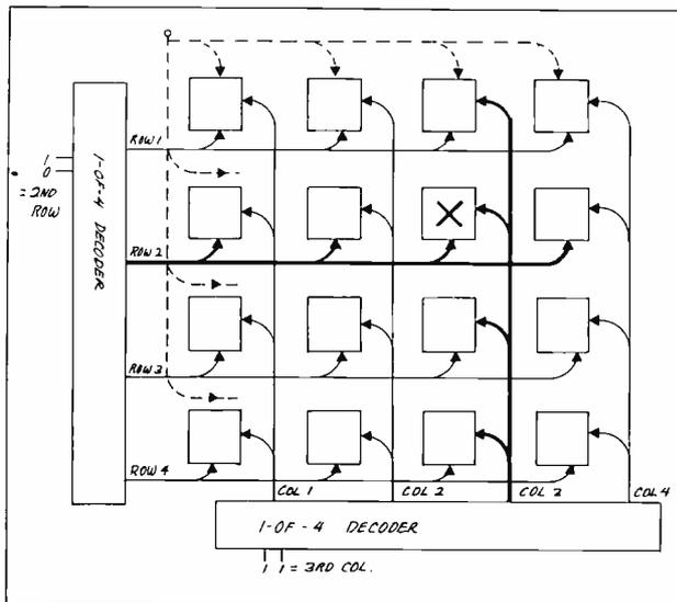
Fig. 10. Sixteen flip-flop memory in  $4 \times 4$  array.
