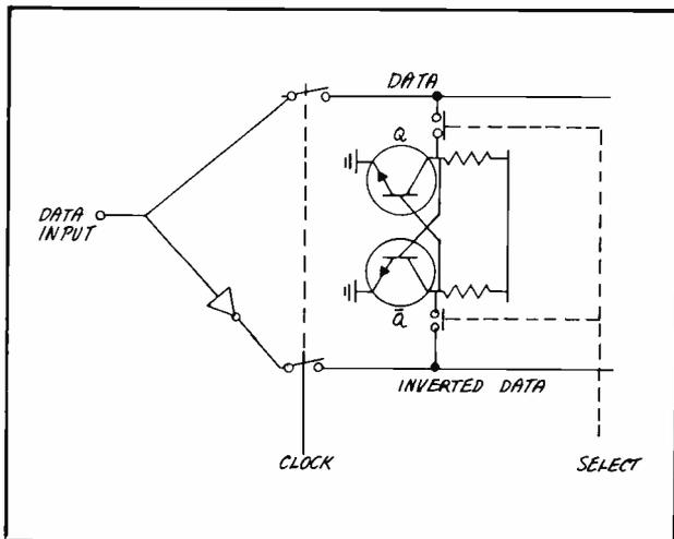
Fig. 6. Flip connected to data and inverted data.
