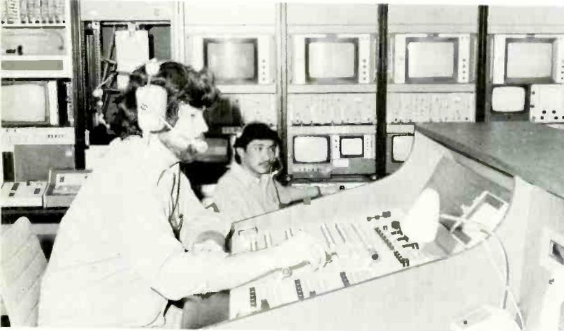
Studio and camera control at Prudential. John Kenlon, producer, is operating Grass Valley 163G switcher. Edward Reyer, systems engineer, is at CCU console.
