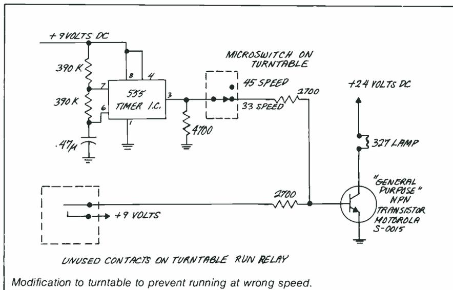
position. A "555" timer circuit supplies a 2 Hz pulse to the base of a "lamp driver" transistor of the turntable run lamp indicator. The turntable run relay supplies a steady DC voltage to the same "lamp driver" transistor when the turntable is running which stops the blinking and the lamp remains on all the time. Stop the turntable, and the lamp resumes blinking until the turntable speed selector switch is restored to the 45 rpm position.
