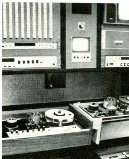
Two views of AHA's studio setup showing IVC one-inch recorders (with TRI editor) and camera control racks.
