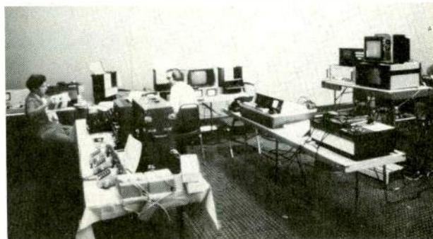
Portable switcher, editors, CCVs, monitors, telephones, etc. in on-location control room.
