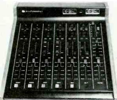
cue, stereo output and stereo monitor output. It has a digital system for start/stop of turntables and tape machines. Under \$1100. ALLEN AND HEATH (U.S. DISTRIBUTOR, AUDIO MARKETING LTD.).
