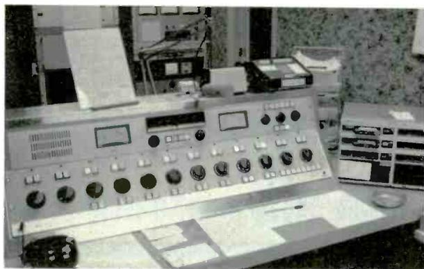
440A Audimax, followed by a 15 kHz Telco line, a CBS 4500 Dynamic Presence equalizer, a UREI 527A 1/3 octave graphic equalizer, and a CBS 4000A Volumax. Limiting is held to about 7 dB.
