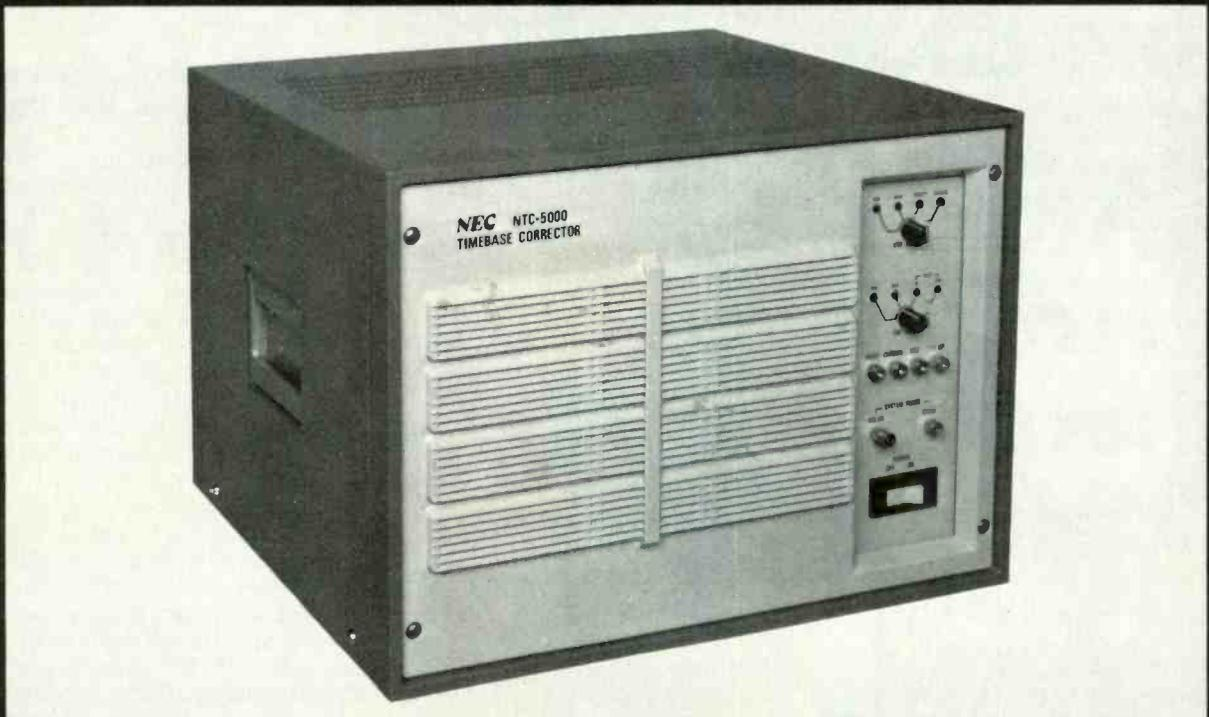
It's the editor's friend. The NEC NTC-5000 is a wide-window time-base corrector with unique, momentary locking circuitry that captures individual color-locked pictures whether the VTR is in pause, rewind or fast-forward modes. So you can zero-in on exactly the frame you want. Fast.
