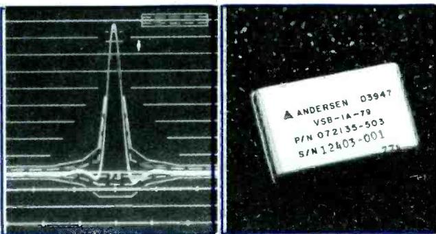
2T test of SAW filter without delay equalization.
