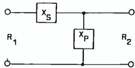
$R_2$  MUST BE GREATER THAN  $R_1$ ,
