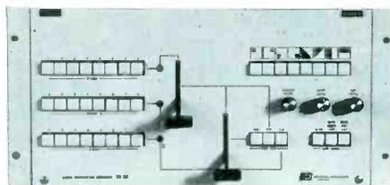
An inexpensive broadcast quality 8-input switcher that features flexibility and ease of operation. Self-contained electronics for rapid installation in ENG and other small mobiles.
