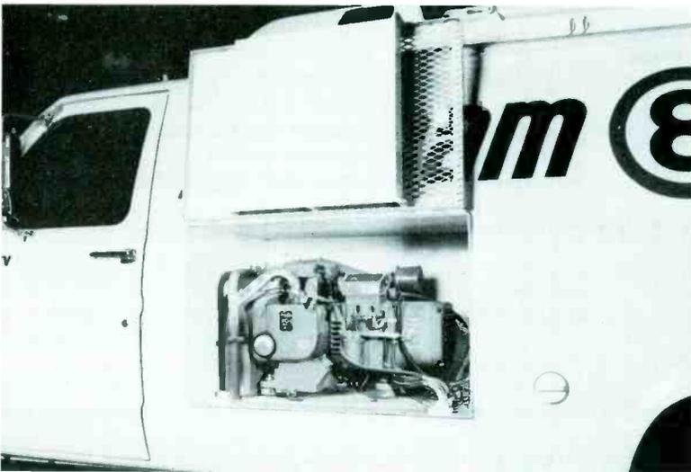
Onan generator provides auxiliary power for van's equipment. External AC power is used when available.
